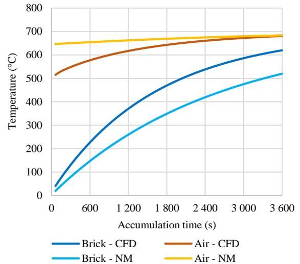
Figure 6 CFD simulation and NM outputs comparison
