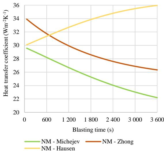
Figure 5 The course of the convective heat transfer coefficient value in the blasting regime
