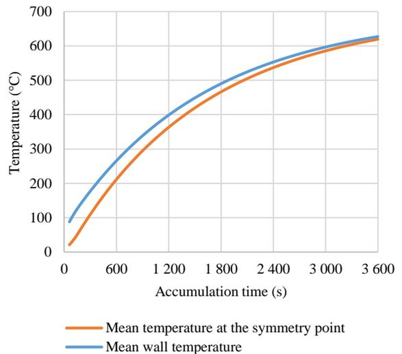
Figure 7 Brick temperature profile during the accumulation
