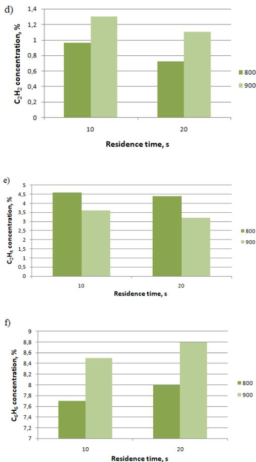
Figure 8 Influence of the residence time on concentration in gas from pyrolysis: a) H<sub>2</sub> b) CO c) CH<sub>4</sub> d) C<sub>2</sub>H<sub>2</sub> e) C<sub>2</sub>H<sub>4</sub> f) C<sub>6</sub>H<sub>6</sub>
