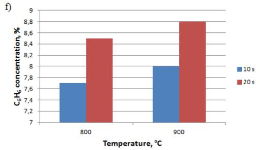
Figure 7 Influence of temperature on concentration in pyrolysis gas: a) H<sub>2</sub> b) CO c) CH<sub>4</sub> d) C<sub>2</sub>H<sub>2</sub> e) C<sub>2</sub>H<sub>4</sub> f) C<sub>6</sub>H<sub>6</sub>
