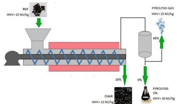
Figure 5 Scheme of RDF Pyrolysis (Polish pilot plant)
