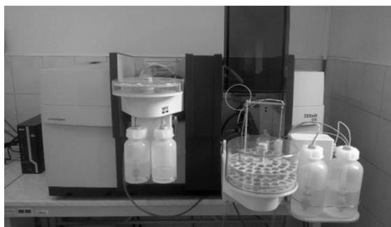
Figure 8 Atomic absorption spectrophotometer by Analytic Jena AG
