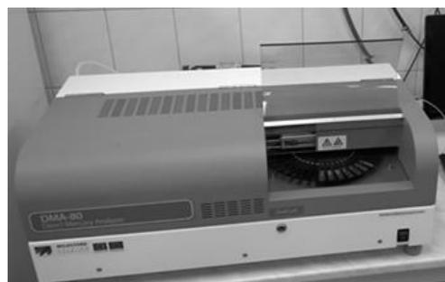
Figure 10 Direct Mercury Analyzer DMA-80 by
