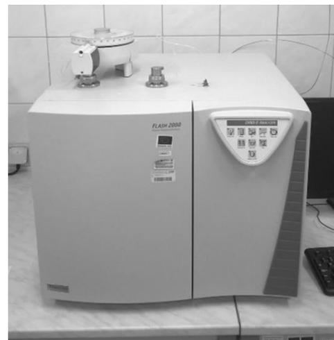
Figure 6 CHNS(O) analyzer Flash 2000 by Thermo Scientific
