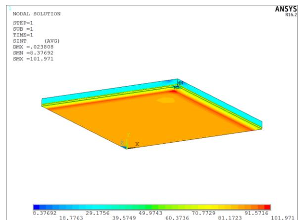
Figure 5 Stress according to Tresca condition at 150°C
