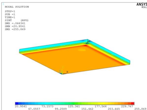
Figure 7 Stress according to Tresca condition at 350°C
