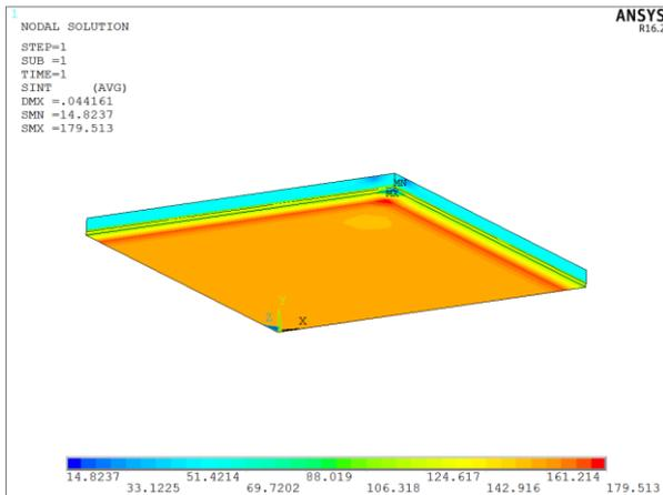
Figure 6 Stress according to Tresca condition at 250°C
