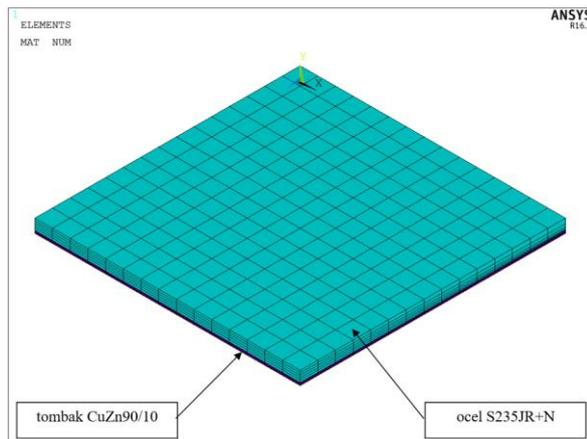
Figure 3 Computational model - finite element network
