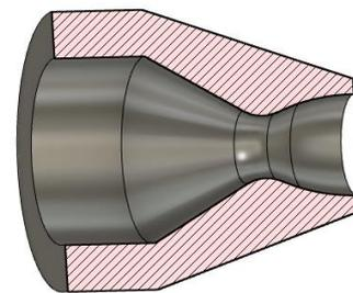
Figure 7 3D design of the minimal length nozzle
