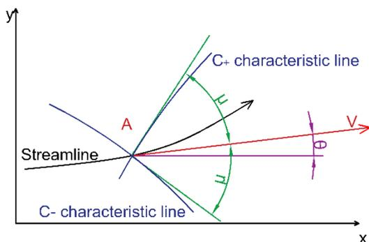
Figure 2 Illustration of left-running and right-running characteristic lines
