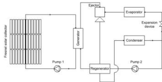
Figure 1 Ejector cooling system with Fresnel solar collector
