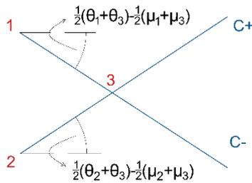
Figure 4 Approximation of characteristics by straight lines
