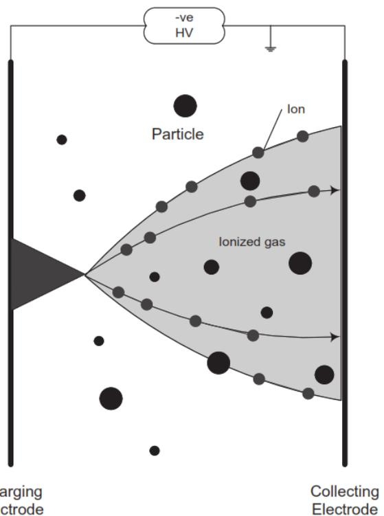
Figure 2 Behaviour of the particles in electrostatic field [10]
