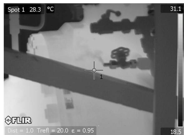
Figure 1 Identification of natural gas leaks.
