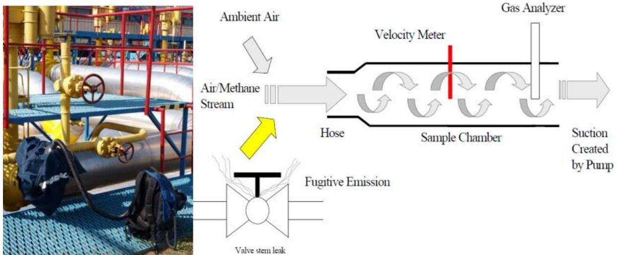
Figure 4 Quantification of methane using the Hi Flow Sampler.
