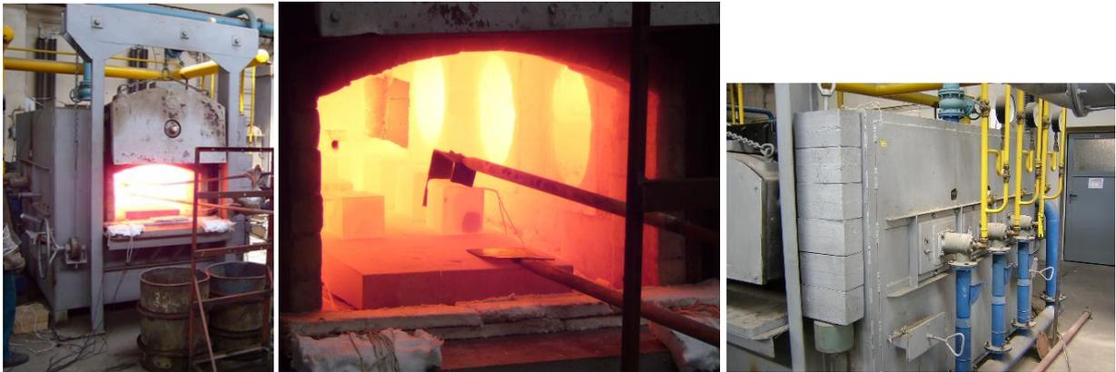
Figure 1 Combustion chamber of heating furnace 5x100 kW
